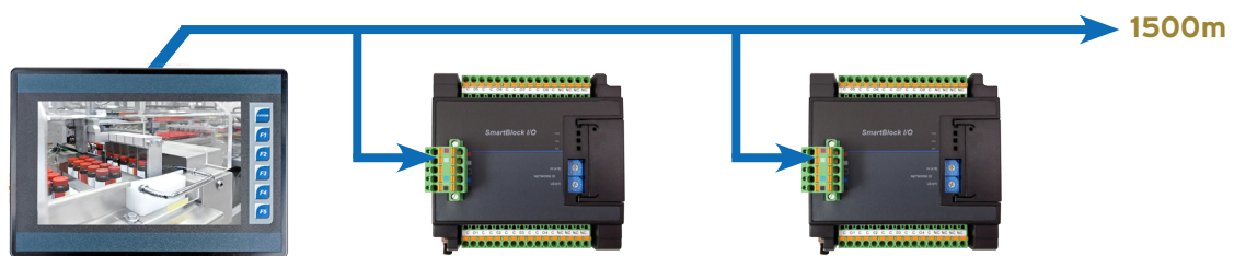
CsCAN supports up to 253 nodes with a maximum network distance of 1500 meters.
