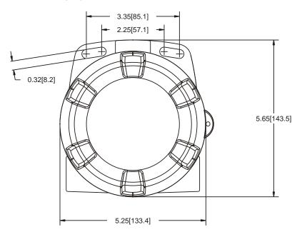
Figure 10. Enclosure Dimensions – Front View
