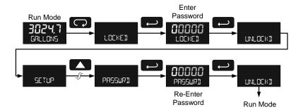
If the correct six-digit password is entered, the meter displays the message LINLOCKI (unlocked) and the protection is disabled until a new password is programmed. If the password entered is incorrect, the meter displays the message LOCKEI for about two seconds, and then it returns to Run Mode. To try again, press Enter while the Locked message is displayed.
