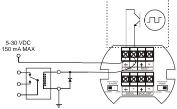
Figure 7. Output Connections
