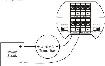
Figure 2. Input Connections without Backlight
