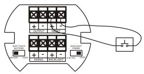
Figure 5. Reset Connections
