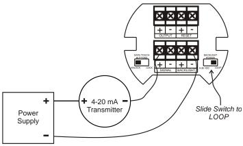
Figure 3. Input Connections with Loop-Powered Backlight
