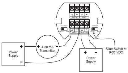
Figure 4. Input Connections with Externally-Powered Backlight
