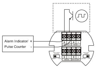
Figure 6. Connection to Device with Internal Pull-Up
