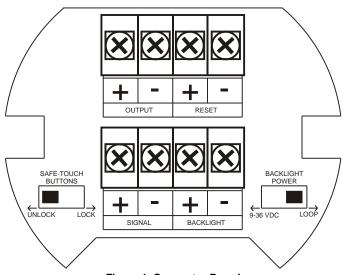
Figure 1. Connector Board
