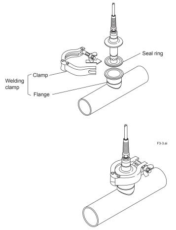
Figure 3.3 Mounted sensor (SC4AJ-SB, -SC)
