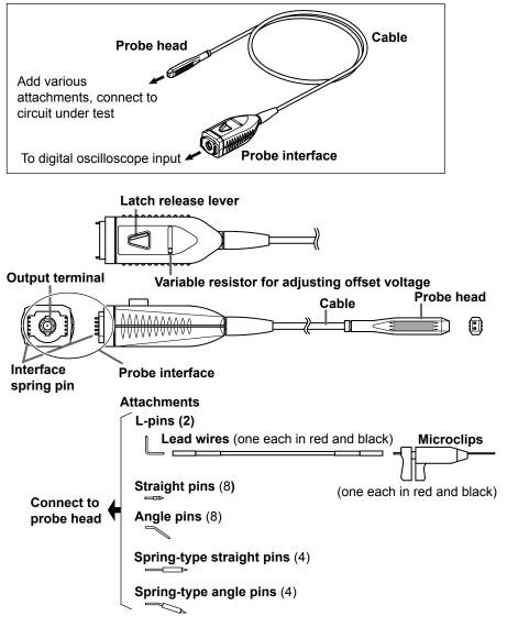
The quantity in parentheses is the number of the various attachments that come with a single probe.
