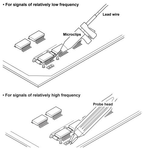
Select an attachment according to the circuit to be tested (straight pin, angle pin, spring-type straight pin, or spring-type angle pin).
