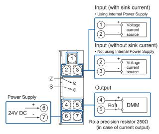
Z: Zero-adjustment volume S: Span-adjustment volume
