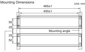
Supplied spacer(50) or Wiring space(30 to 60)
