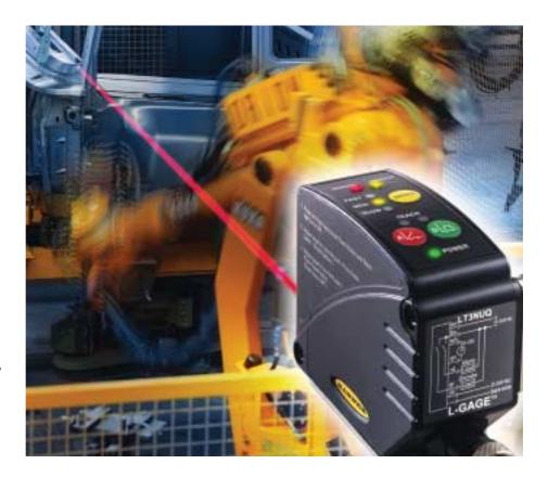
The LT3 uses pulsed time-of-flight technology to achieve unsurpassed performance. The laser pulses one million times per second. The microprocessor records the time required for each pulse to travel to the retro-reflective target and back to the sensor. Every millisecond, it averages one thousand pulse times and outputs a value from the microprocessor.
