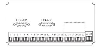
\* 8 VDC Power supplied on Pin 9 to power modem or two way pager
