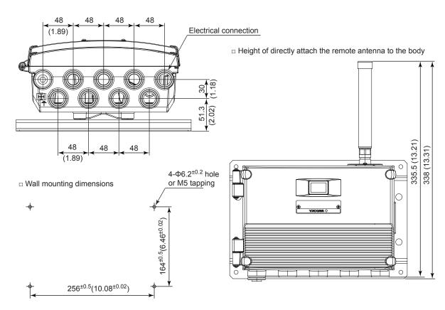
If not specified, the tolerance is  $\pm 3\%$ . However, in cases of less than 10 mm, the tolerance is  $\pm 3$  mm.
