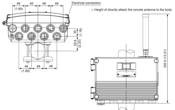
If not specified, the tolerance is ±3%. However, in cases of less than 10 mm, the tolerance is ±3 mm.
