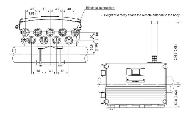
If not specified, the tolerance is  $\pm 3\%$ . However, in cases of less than 10 mm, the tolerance is  $\pm 3$  mm.
