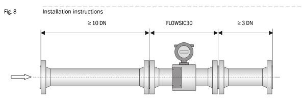
In order to achieve the specified meter accuracy, ensure 10D of straight inlet and 3D of straight outlet pipe length as a minimum.
