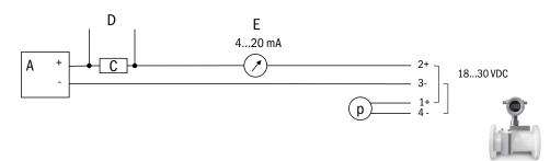
Fig. 16 Non-intrinsically safe installation, HART<sup>®</sup> + Modbus RS485 output
