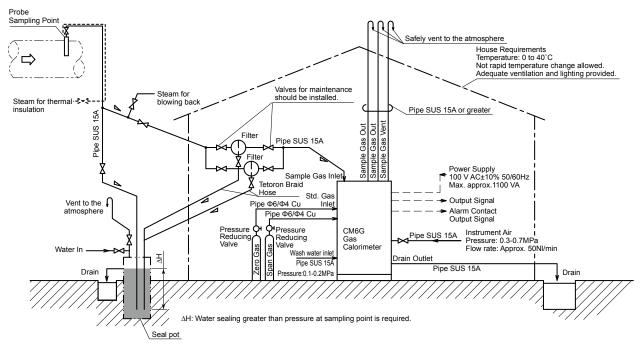
(9) Locate the standard gas cylinders at the place where they are not exposed to direct sunshine and comparatively cool.
