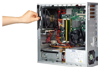
Gently press the hook to pull the air filter out
