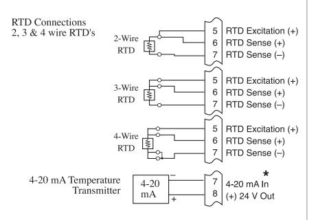
\* Or optional steam trap monitoring input in some saturated steam applications.
