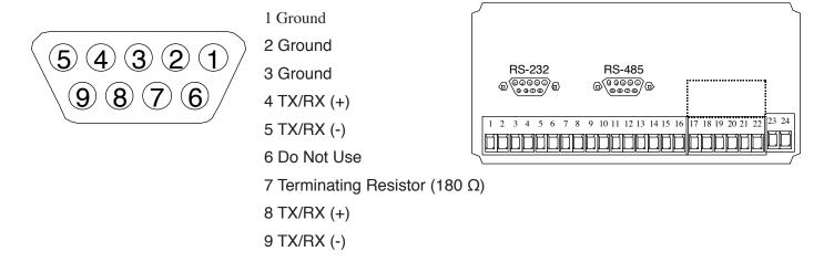
**NOTE:** To termintae cable end, connect Pin 7
