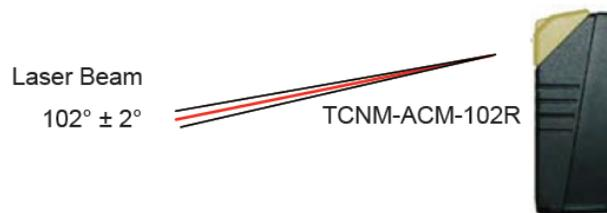
Laser Beam Output Position
