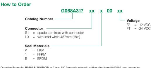
Ordering Example: R068A317S1E00F1 = 2-way NC (normally closed), orifice size 2mm (0.079in), pad-mounting body width 22mm (0.867in), spade terminals with connector, EPDM seals, 24 VDC
