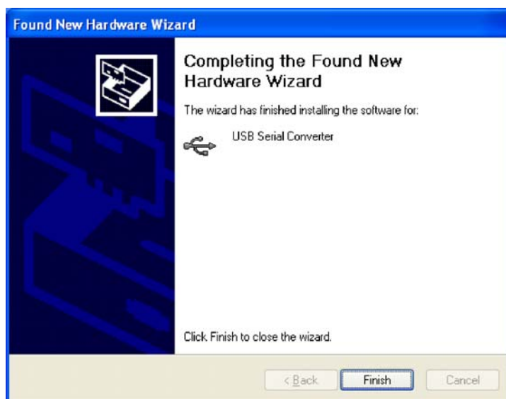
Fig. 4.1: Installing the USB driver
