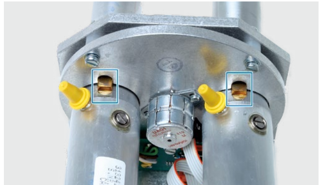
Cell with locking function for simple mounting
