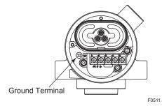
Figure 5.11 Ground Terminal inside the Terminal Cover
