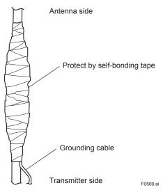
Figure 5.9 Surge Protective Device Protection by Self-bonding Tape
