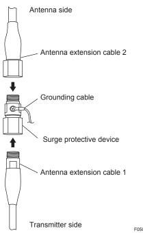
Figure 5.8 Connection of the Surge Protective Device and Antenna Extension Cable
