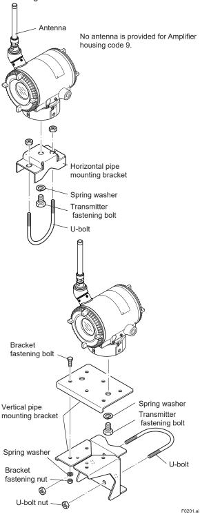
Figure 2.1 Transmitter Mounting Hardware
