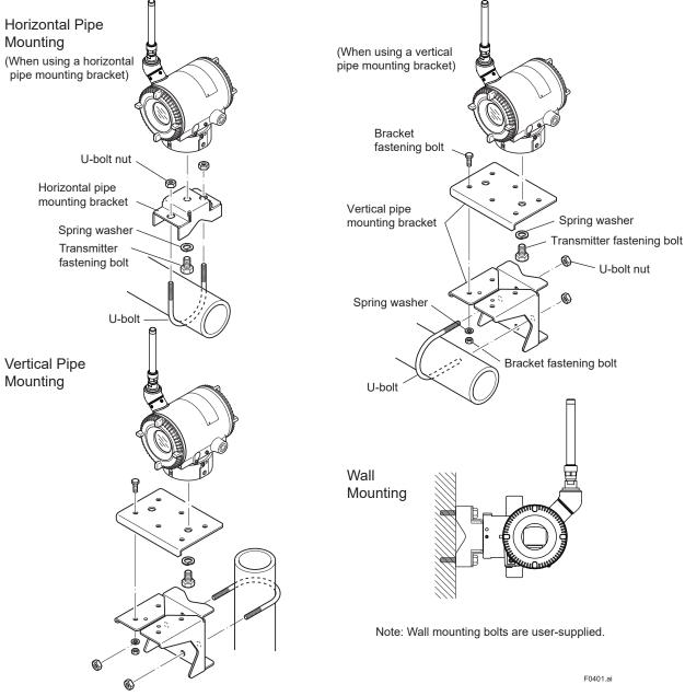
Figure 4.1 Transmitter Mounting
