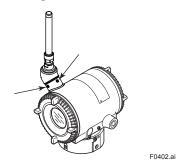
Figure 4.2 Mounting Screw Position
