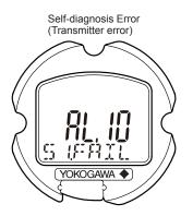
Figure 7.4 Error Check with Integral Indicator
