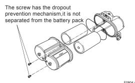
Figure 8.4 Disassembling the Battery Pack
