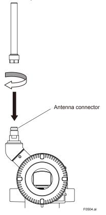
Figure 5.4 Mounting the Antenna
