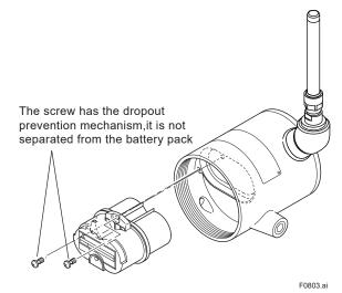
Figure 8.3 Removing the Battery Pack
