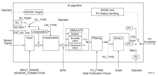
Figure 9.1 Example schema of analog input object
