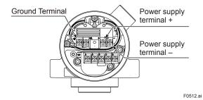
Figure 5.12 Connection of External Power Source Terminal
