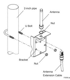
Figure 5.6 Fixing the External Antenna
