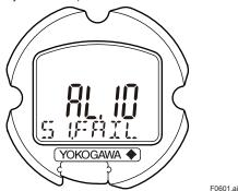
Figure 6.1 Integral Indicator with Error Code
