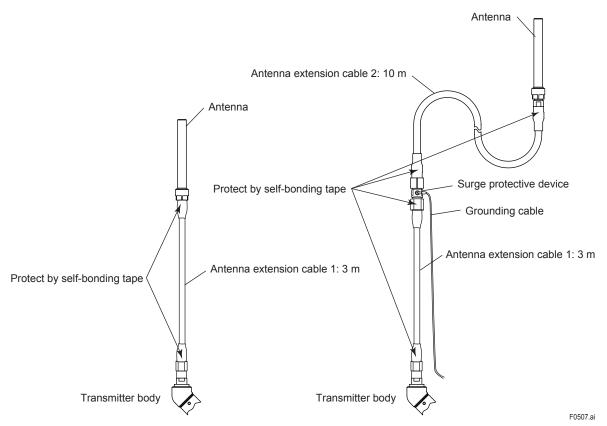
Figure 5.7 Wiring the Antenna Extension Cable
