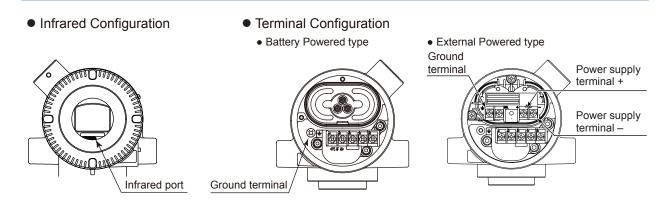
• Terminal Wiring Example for the External Power Source Terminal
