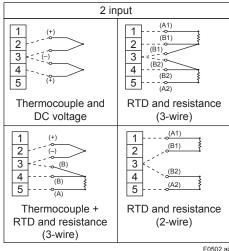
Figure 5.2 YTA510 Input Terminal Wire Connection Diagram
