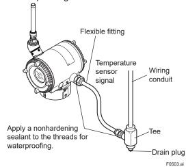
Figure 5.3 Example of Wiring Using a Wiring Conduit
