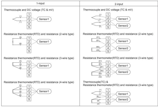
Figure 7.2 YTA510 Wire Connection Diagram
