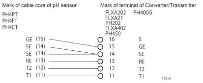
Note: 2 cable cores of pH sensor should be connected to the terminal of Converter/Transmitter 14 (SE). There is no wire connection to Converter/Transmitter 16 (S).
