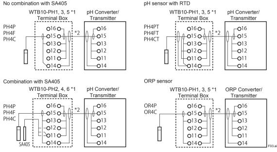
\*1: Terminal box is used only where pH/ORP transmitter is installed remotely from pH or ORP sensor (normally not needed). Refer to Table 2 for WTB10 type.
