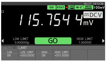
Figure 2.18 Example of LIMIT calculation result display
