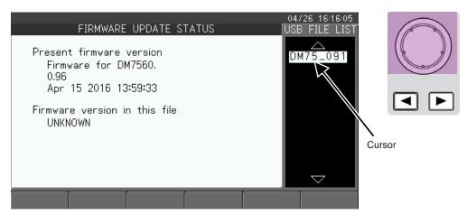
5 On the SOFTWARE UPDATE STATUS screen below, the upper file information indicates the current software of this instrument and the lower information indicates the update file. Check that the file is normal.
