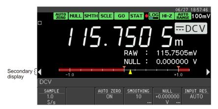
Figure 2.16 Example of secondary display
