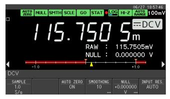
Figure 2.17 Example of ANALOG METER display
