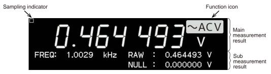
Figure 2.11(a) Example of NUMERIC display (FONT: 7SEG)
