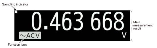
Figure 2.11(d) Example of NUMERIC display (FONT :NORMAL)
