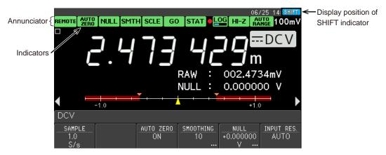
Figure 2.9 Example of annunciator and indicators
