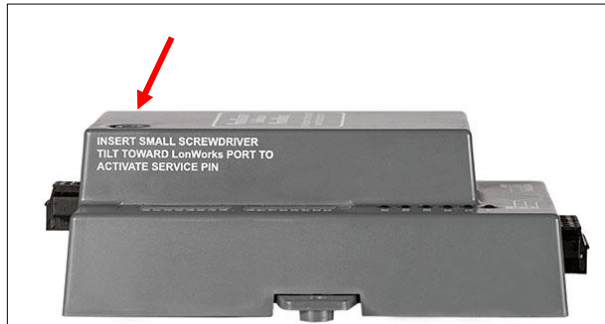
Figure 26: LonWorks Service Pin Location
