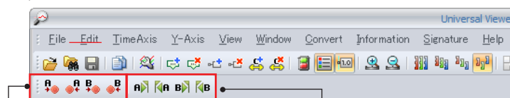
Move the cursor to the alarm change point. Move the cursor to a mark.
