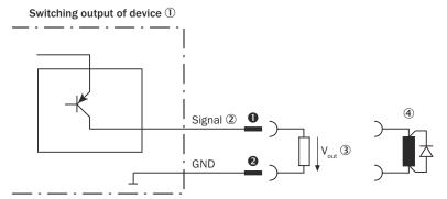
Figure 15: Wiring a digital output
