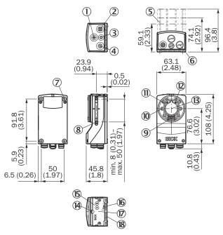
Figure 3: structure and device dimensions, unit: mm (inch), decimal separator: period
