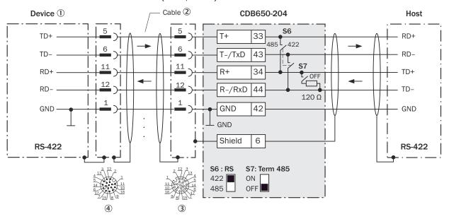
Figure 22: Wiring data interface RS-422 of the device in the connection module CDB650-204
