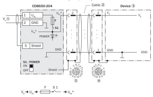
Figure 20: Connecting supply voltage for the device in CDB650-204 connection module
