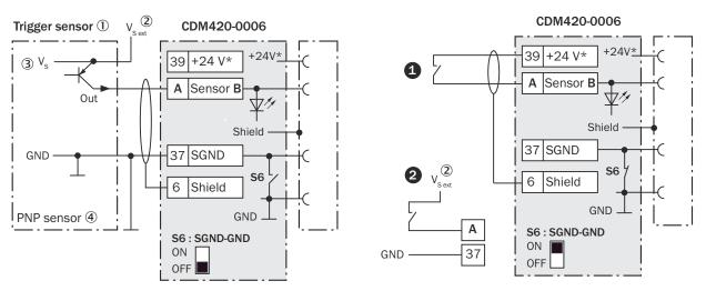
Figure 37: Left: Trigger sensor connected potential-free and supplied with power externally. Right: Alternatively switch, **0** supplied with power by connection module CDM420-0006 or @connected potential-free and supplied with power externally. Switch setting S6 then as in left figure.
