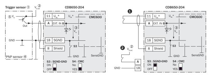
Figure 27: Left: Trigger sensor connected potential-free and supplied with power externally. Right: Alternatively switch, **1** supplied with power by connection module CDB650-204 or **2** connected potential-free and supplied with power externally. Switch setting S3 then as in left figure.
