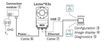
Figure 12: Connection block diagram
