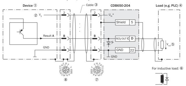
Figure 28: Wiring the digital outputs "Result 1" to "Result 4" of the device in the connection module CDB650-204
