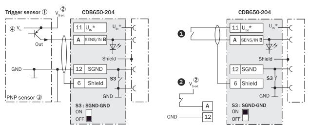
Figure 25: Left: Trigger sensor connected potential-free and supplied with power externally. Right: Alternatively switch, # supplied with power by connection module CDB650-204 or @connected potential-free and supplied with power externally. Switch setting S3 then as in left figure.
