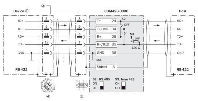
Figure 34: Connecting data interface RS-422 of the device in the connection module CDM420-0006
