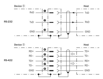
Figure 14: Wiring of the serial data interfaces RS-232 and RS-422
