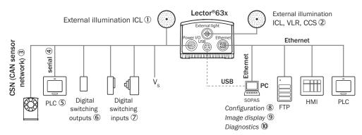
Figure 13: Facilities for connecting
