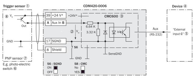
Figure 38: Trigger sensor supplied with power by connection module CDM420-0006
