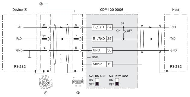
Figure 33: Connecting data interface RS-232 of the device in the connection module CDM420-0006
