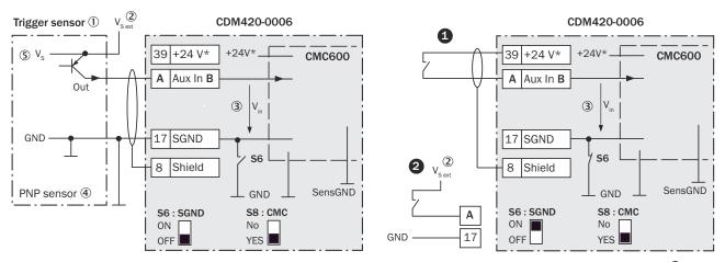
Figure 39: Left: Trigger sensor connected potential-free and supplied with power externally. Right: Alternatively switch, **1** supplied with power by connection module CDM420-0006 or **2** connected potential-free and supplied with power externally. Switch setting S3 then as in left figure.
