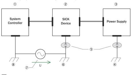
Figure 11: Example: Prevention of equipotential bonding currents in the system configuration by the insulated mounting of the device
