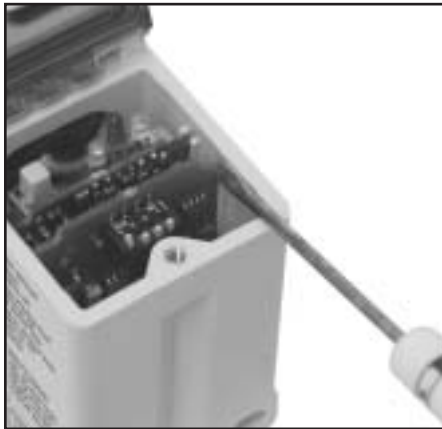
Figure 2. Remove the output card using a small screwdriver to dislodge it from its connector.
