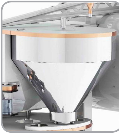
Q60AFV adjustable-field sensors are used to measure bread mix inside highly polished stainless steel hoppers
