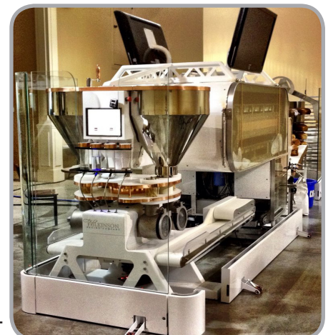
View of the Bread Bakery with dry ingredient hoppers, water and mixing chambers displayed
