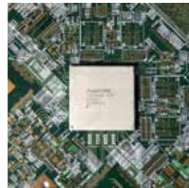
The fast ScopeCORE internal processor
