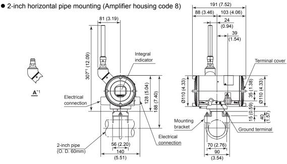
\*1: When amplifier housing code 9 is selected, the value is 187 mm (7.36 inch). In this case, the figure is shown as A.
