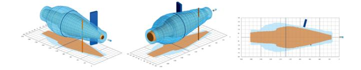
The infinitely and individually adjustable detection range is the optimal solution for your application. If the ambient conditions change, the sensor can be quickly and easily adjusted to the new requirements. Thanks to the Connect+ software or the SOPAS Engineering Tool from SICK, there are practically no limits to the adjustment options.
