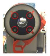
2. Remove the black insert and set aside (store in the shipping box of the protection window for further use)..
