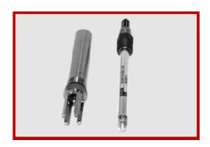
17. Slide the electrode into the protection tip and thread the PG13.5 connector in place.
