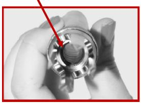
6. If you are using a PG13.5 electrode, proceed to <u>Step 15</u> for complete installation. For Yokogawa Y-Cap electrodes, take the smallest of the (3) O-rings (C) provided in the bag with the Instruction Manual.
