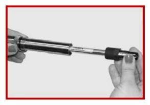
18. Once the electrode it tightened in place, take the largest O-ring (A) that is provided in the bag with the Instruction manual, and place it on the protection tip below the threads and next to the knurled finger grip.
