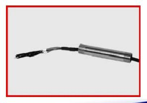
13. Once the cable is threaded thru the metal tube attach the cable to the sensor and screw the metal tube and the sensor tip together as seen here.
