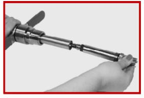
Locate the metal process connection. There are two different types of threads on the adapter. One side is a 1.25" NPT thread and the other is a Gas straight thread.
