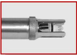
15. Steps 15 - 20, are for installing a sensor with a PG13.5 connection into the PR10. You should have the following parts, the electrode, the sensor tip from the PR10 holder and the metal tube provided in the bag with the manual.
