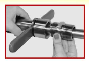
The side that contains a bevelled end on the inside has the Gas straight thread **(A)**, where the side that is flushed has the NPT thread **(B)**.
