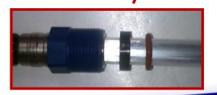
16. Set aside the metal tube that comes in the bag with the manual it will not be used. You will just be using the sensor tip from the PR10 holder and the electrode with the PG13.5 connection.
