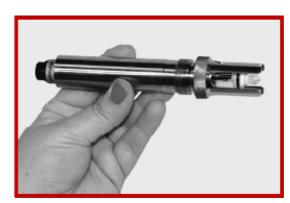
10. Take the electrode tip and the largest O-ring (A) that is provided in the bag with the Instruction manual, and place it on the protection tip below the threads and next to the knurled finger grip.
