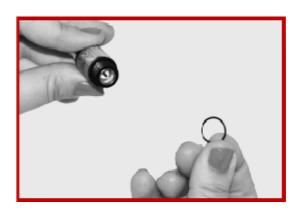
7. Place the O-ring on the electrode below the threads of the cable connector as show in the image.
