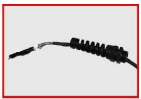
23. Thread the two pieces of the cable strain relief together. Thread the cable strain relief into the PR10 holder.
