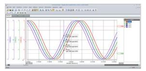
• Viewer function: Waveform display, digital display, circular display, list display, report display, operation log display, waveform superimposed display, etc.
