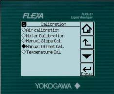
If you perform the Air calibration it will read around 95-100% in air before the calibration and around 110-115% after the calibration. This is why the *Manual Slope Calibration* is required instead.
