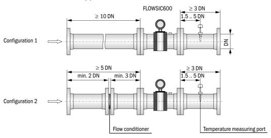
Two straight pipes are to be installed in the inlet and outlet sections if the meter is to be used bidirectionally. The temperature measuring point is to be located downstream of the FLOWSIC600, seen in the direction of predominant use. The temperature measuring point must not be installed more than 8 DN from the meter.
