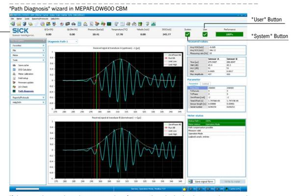
If the zero phase values do not meet the aforementioned criteria, the zero phase needs to be adjusted according to angepasst werden (see Technical Information).
