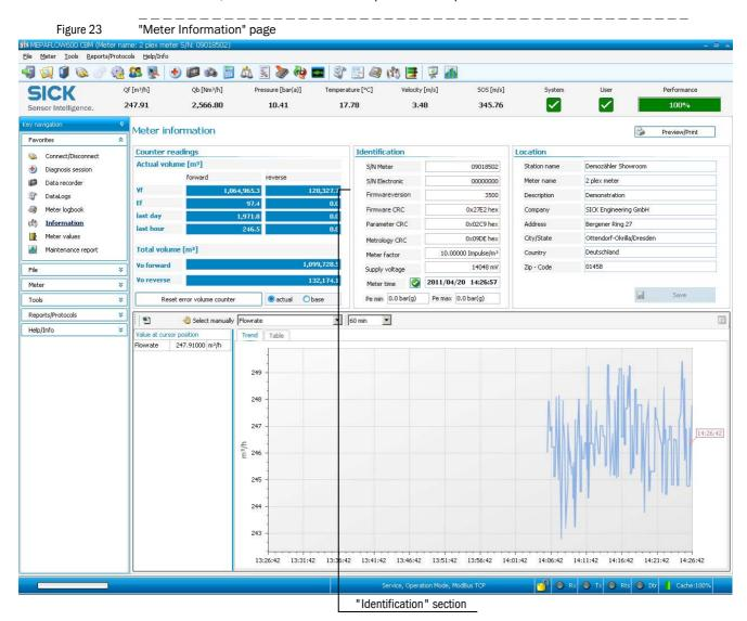
The FLOWSIC600 firmware is stored on a non-volatile memory (FLASH PROM). The program code for the signal processor and system micro-controller are identified by a version number (Reg. #5002 "FirmwareVersion") and a check sum (Reg. #5005 "ProgramCRC") and can be verified as mentioned above.
