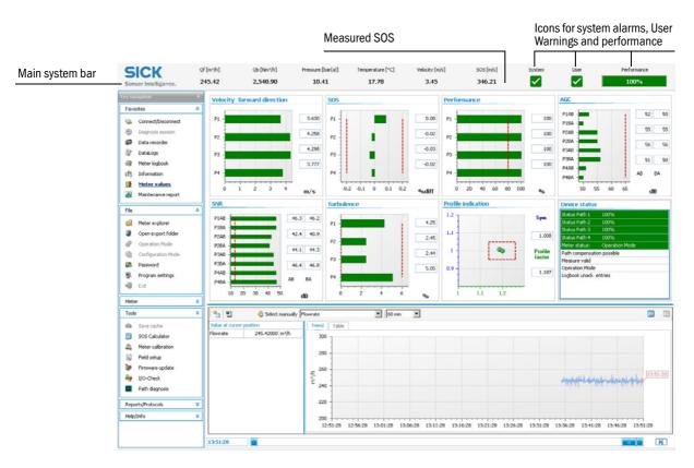
All entries in logbooks or datalogs saved in the meter's memory (FRAM) are written with a time stamp containing the meter time. The meter time can be synchronized with a master clock (e.g. PC clock) via MODBUS or with MEPAFLOW600 CBM.
