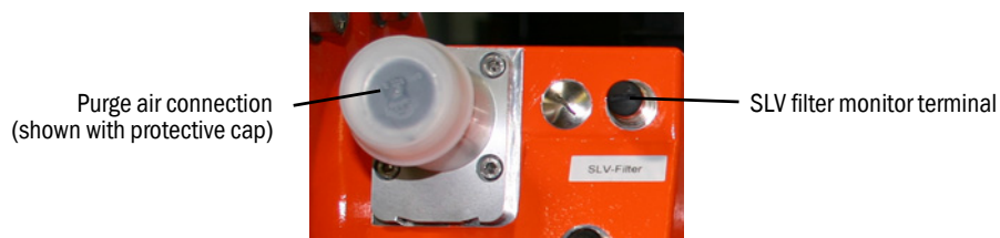
Fig. 22: Connection of the purge air supply
