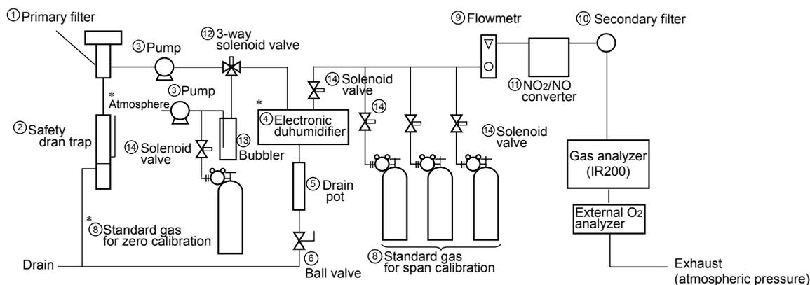
\*A dehumidifier must be used for NO, SO<sub>2</sub>, and CO (0-200 ppm) measurements (to prevent saturation at 28°C). Use either atmospheric air or cylinder gas as a zero calibration gas and supply it through a bubbler (humidifying) to reduce interference of water.
