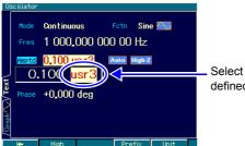
Select the userdefined unit When the input field of the desired parameter is open, place the cursor over the right-most unit and change the unit with the  $\bigcirc$   $\bigcirc$  up/down arrow keys or the  $\bigcirc$  modify knob. The unit name that is displayed can be freely set. Even if the unit is changed, only the display unit changes, and the actual output values remain unchanged.
