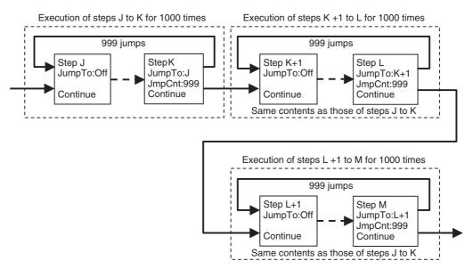
Steps with the same contents can be created easily by using the [Copy] and [Paste] soft keys. Create the steps with the same contents then revise only the required portions.
