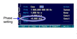
If the waveform of the previous step is DC or noise, oscillation in the next step starts from phase 0°.
