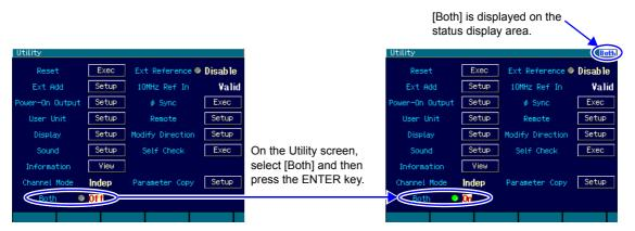
On screens other than the Utility screen, the function can be switched on/off by pressing the [CH1/CH2] key for at least 2 seconds.
