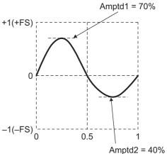
Note that when the respective amplitudes are changed, the top and bottom peak values of the waveform change.
