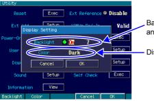
Backlight on/off and brightness Set backlight on/off and the brightness when the backlight is on.
