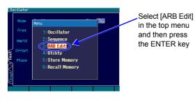
Press the WEND MENU key to display the top menu window. In this window, select [ARB Edit] and then press the ENTER ENTER key to open the ARB Edit screen.
