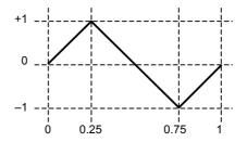
**1.** When the [New] soft key is pressed and the number of control points is set to 2, the following setting results.
