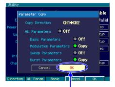
Select [OK] and then press the ENTER key to execute copying. 4. Once the above settings have been completed, select [OK] at the bottom of the window and then press the ENTER key to execute copying.
