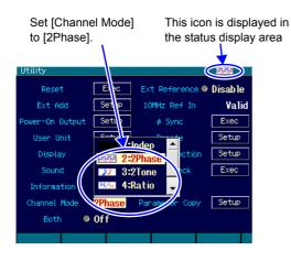
On the Utility screen, set [Channel Mode] (channel mode) to [2Phase] (2-phase) (normally, [Indep] (independent) is set). As a result, 2-phase oscillation is set.
