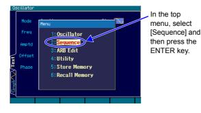
Press the <u>MENU</u> Key to open the top menu window. In that window, select [Sequence] and then press the <u>ENTER</u> ENTER key to switch to the sequence oscillation mode.
