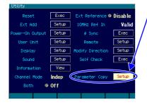
On the Utility screen, select [Parameter Copy] and then press the ENTER key.  On the Utility screen, select [Parameter Copy] and then press the ENTER key.
