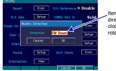
Item transition direction during clockwise rotation Select whether the selected items move downward or upward as the modify knob is rotated clockwise (CW) with the choice list of the oscillation mode or the waveform displayed.
