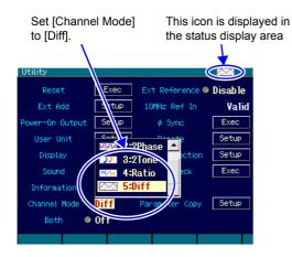
On the Utility screen, set [Channel Mode] (channel mode) to [Diff] (differential) (normally, [Indep] (independent) is set). As a result, differential output oscillation is set.
