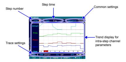
[PRM] and [SCL] displayed in the trace settings indicate the display item and the height of the trace frame, respectively. [OFS] indicates the bottom values in the trace frame for frequency, amplitude, and duty, and the center value in the trace frame for the offset and phase.
