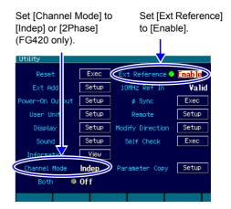
Check that all the slave units operate with the external frequency reference. If the [Ref] icon in the status display area at the top of the screen is displayed without blinking, this indicates operation at the external frequency reference.
