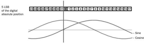
Codification magnetic tape TTK70 The absolute coding of the magnetic tape allows a maximum
