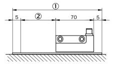
0 Required band length = measurement path + 80 mm 2 Measurement path
