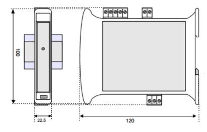
Dimensions in inches are 0.89"W x 3.94"H x 4.72"D Note: Number of I/O terminal connections varies from model to model
