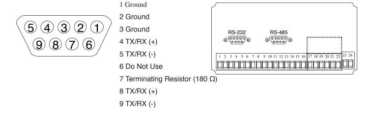
**NOTE:** To terminate cable end, connect Pin 7 to either Pin 4 or Pin 8.
