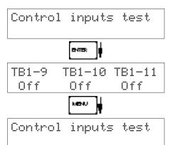
Press Enter to test the control inputs.
