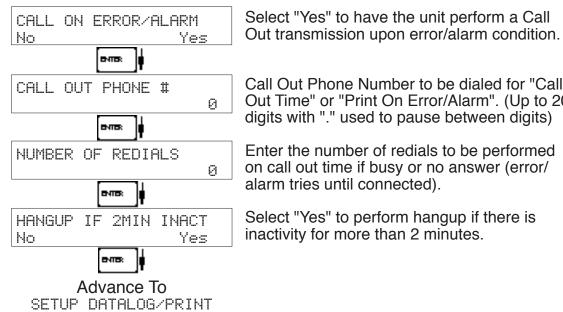
Call Out Phone Number to be dialed for "Call Out Time" or "Print On Error/Alarm". (Up to 20 digits with "." used to pause between digits)
