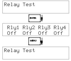
Press Enter to test the relays.
