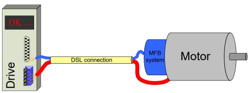
Figure 1: Drive system with HIPERFACE DSL®
