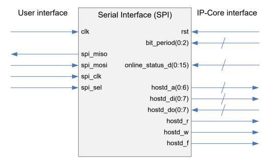
Figure 50: Serial interface block signals
