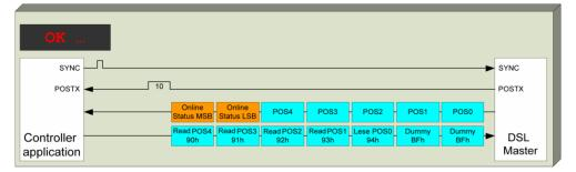
Figure 24: Polling registers for the fast position in SYNC mode
