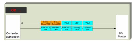
Figure 22: Polling of rotation speed registers in free running mode
