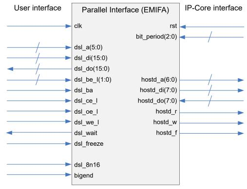
Figure 52: Parallel interface block signals
