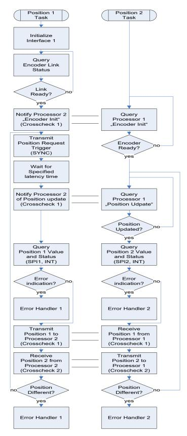
Figure 39: Tasks Position 1 and Position 2
