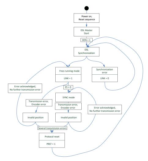
Figure 19: Status table for DSL system start.
