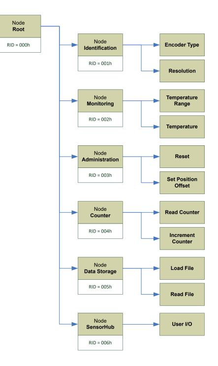
Figure 44: Tree structure of the resources database
