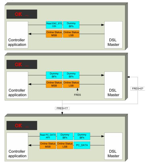
Figure 28: Reading from remote register
