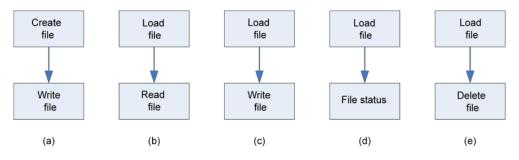
Figure 46: Workflows for data storage
