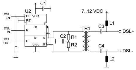
Figure 6: Interface circuit with two core cable (integrated in cable)
