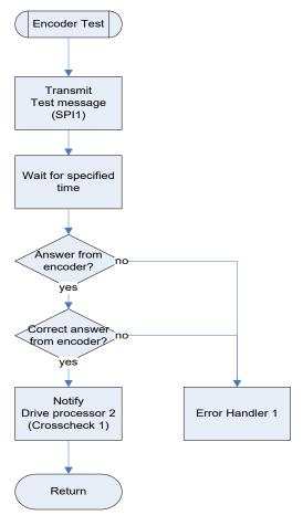
Figure 42: Task Encoder Test
