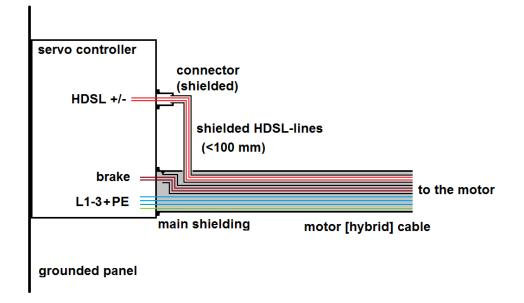
Figure 56: Connection of the hybrid motor cable to the servo controller
