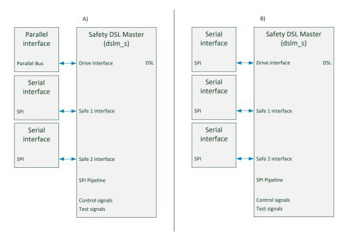
Figure 49: Combination of interface blocks
