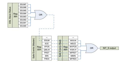
Figure 17: Interrupt masking
