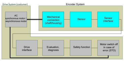
Figure 35: General view of a servo feedback loop
