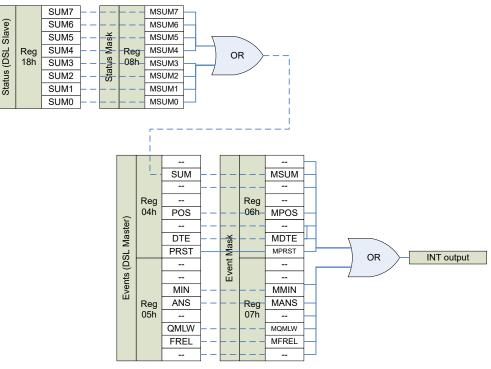
Figure 15: Interrupt masking
