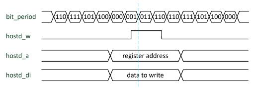
Figure 55: Write access basic interface
