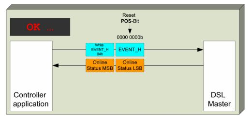
Figure 32: Acknowledgment of event bits
