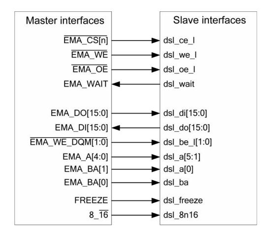
Figure 53: Allocation of parallel interface block to host
