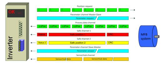
Figure 3: Data channels in HIPERFACE DSL®
