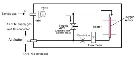
Note: If no suction device [-N] is specified, the aspirator is removed from this diagram.
