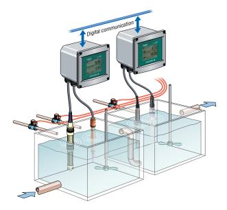
For dual sensor measurement, the combination of two same type sensor inputs -pH/ORP and pH/ORP (analog sensor only), SC and SC, and DO and DO - are available.
