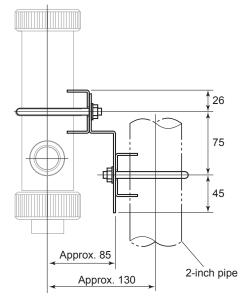
Bracket (thickness : 3) U-bolt holes for holder mounting 756-ø10 holes  $70\pm0.3$ 92Holes dimension for wall mounting
