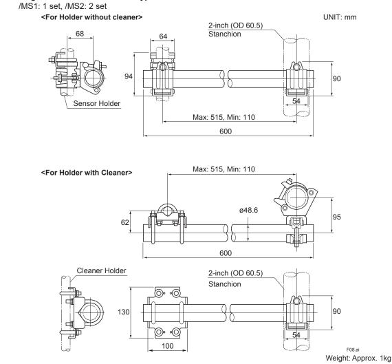
Stainless Steel Mounting Bracket for Submersion Type Holder /MS3: 1 set, /MS4: 2 sets
