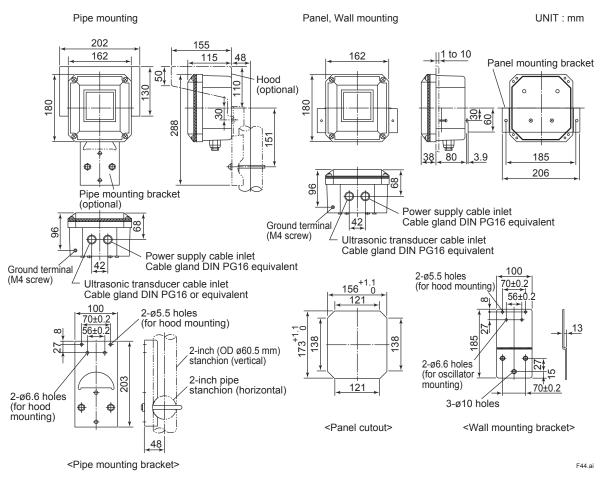
External dimensions of additional noise filter assembly when PUS400G-NN-KC
