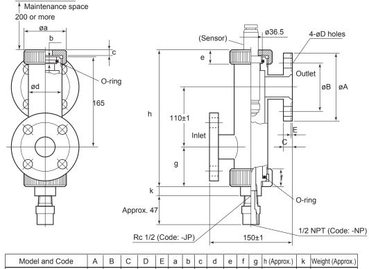
Flow-Through Type Holder (For MLSS Meter), With Jet Cleaner (See separate drawing for mounting bracket) FH350G UNIT : mm
