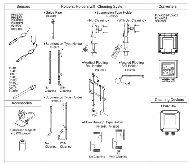
System Configuration (General Purpose, Non-Explosionproof Types)
