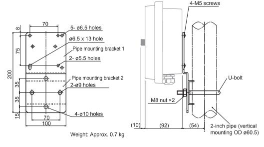
• Wall or Panel mounting bracket for additional noise filter assembly (option code: /W, /PA) UNIT : mm
