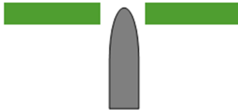
Figure 8 The Pins' tips should be visible through the conductive rings, to ensure proper pin detection during inspection. The pin tips should not extend too much beyond the board surface.
