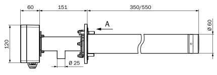
FLSE100-PM and FLSE100-PH sender/receiver units
