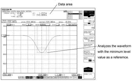
Notch width measured waveform (PEAK)
