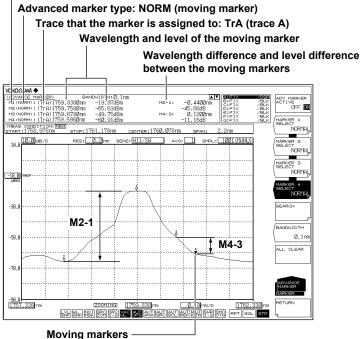
A number is displayed with the moving marker. When active, the marker is solidly filled.
