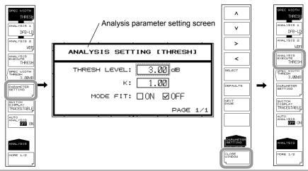
If you only want to change the THRESH LEVEL, you can also do so with the SPEC WIDTH THRESH soft key.
