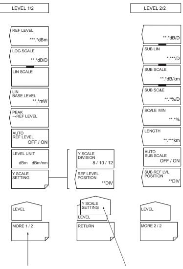
The LEVEL soft key menu is split into two parts. This key switches between the menus. In addition, in some cases this may change to a function that closes the window. For example, when the MORE 1/2 soft key is pressed, the menu changes to the LEVEL 2/2 soft key menu, and the key display changes to MORE 2/2.
