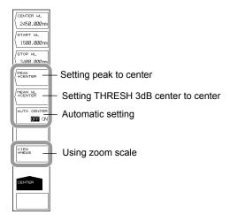
Also, you can set the wavelength of the moving marker placed on the measured waveform as the center wavelength (frequency / wavenumber).
