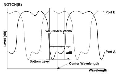
Obtain the width (xdB\_Notch\_Width) between the two points, which are above the bottom level of each channel by the parameter THRESH\_LEVEL, and its center wavelength (Center\_Wavelength).
