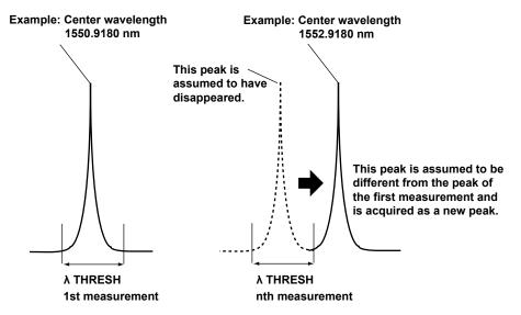
Channel matching range (e.g. λ THRESH = ±1.00 nm) 1549.9180 nm to 1551.9180 nm
