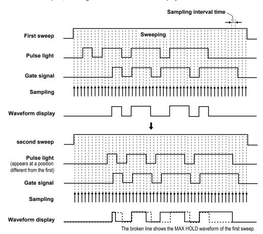
Because the AQ6376 does not show data that is sampled when the gate signal is inactive, the wavelength data during this period may be missed, but because the sampling time and gate signal (pulse light) are asynchronous, performing repeat sweep using the MAX HOLD function eventually results in all the waveform data in the span range to be shown.
