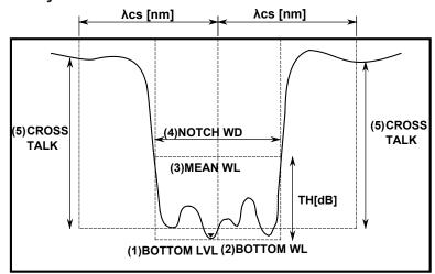
(1) Bottom level (BTM LVL): Value of level at the waveform bottom position(2) Bottom wavelength (BTM WL): Value of wavelength at the waveform bottom
