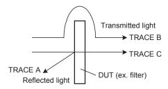
(2)Estimating the reflectivity (trace C) from the transmission light spectrum (trace A)
