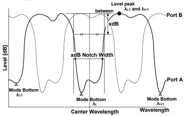
Obtain the width (xdB\_Notch\_Width) between the two points, which are below the higher point of either the left peak level or the right peak level of each channel by the parameter THRESH\_LEVEL, and its center wavelength/frequency (Center\_Wavelength).
