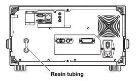
The recommended purge gas flow rate into the AQ6376 is 15 to 20 SCFH (7 to 9.5  $\rm L/min$ ).
