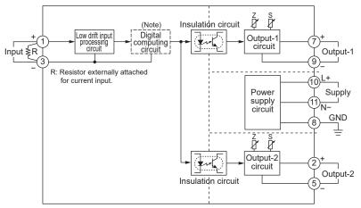
Note: Digital computing circuit is added for the input/output suffix codes other than "A" and "6".
