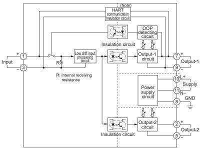
Note: The HART communication isolation circuit is added when the option code / HC is specified.
