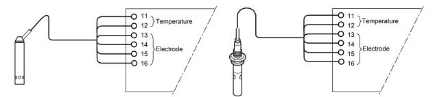
SC4AJ Conductivity Sensor (two-electrode system) Applicable Converter / Transmitter: SC450G, FLXA202/FLXA21, SC202G, SC202SJ For SC100, see SD12D11A01-01E. SC8SG Conductivity Detector (two-electrode system, four-electrode system) Applicable Converter / Transmitter: SC450G, FLXA202/FLXA21, SC202G, SC202SJ
