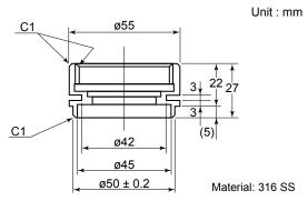
Note: If you make the welding socket for screw-in type, refer to the above drawing.
