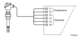
SC210G Conductivity Detector (two-electrode system) Applicable Converter / Transmitter: SC450G, FLXA202/FLXA21, SC202G, SC202SJ
