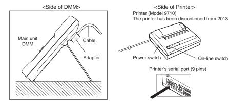
Infrared (IR) Adapter and RS-232 cable
