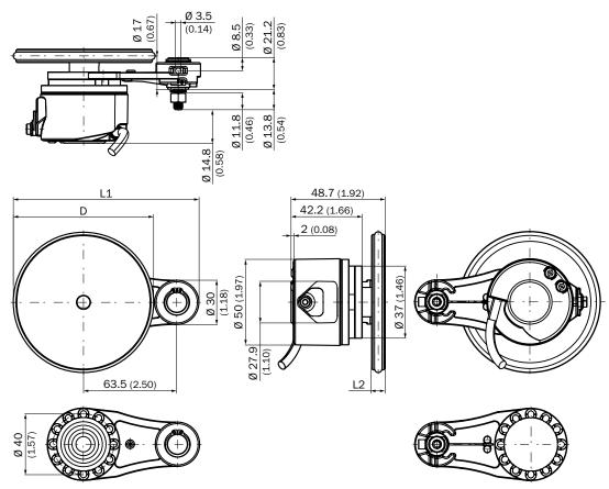
Single wheel, 63.5 mm spring arm, wheel on mounting side, connector
