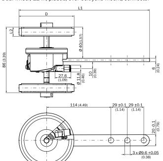
Dual wheel, 12 in, plastic, over-belt yoke mount, connector, cable connection
