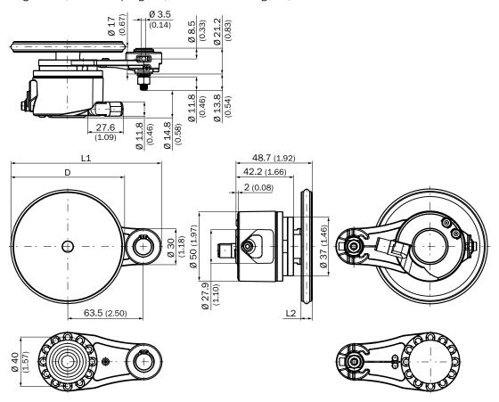
Single wheel, 63.5 mm spring arm, encoder on mounting side, cable conntection
