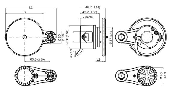
Dual wheel, 12 in, plastic, over-belt yoke mount, connector
