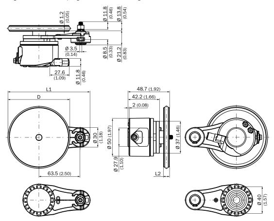
Single wheel, 63.5 mm spring arm, wheel on mounting side, cable connection
